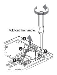
5 Insert the new lamp all the way in until it is securely in place (1). Tighten the two screws (3). Fold down the handle to replace it (2).
