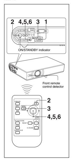
1 Plug the AC power cord into a wall outlet.
