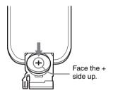
**3** Put the lithium battery holder back into the Remote Commander.
